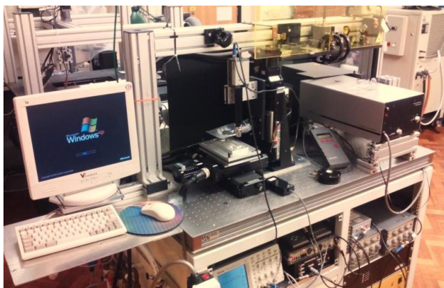
Fig. 1. CO 2 laser-based micro-machining system used for processing Borofloat ® 33 glass.
