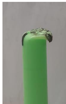
Figure 7. Side view of worn pin slid at 0.81 m/s
