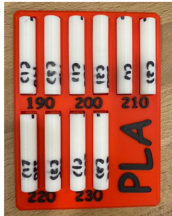
Figure 2. FDM 3D printed PLA pin specimens. Each individual pin is labelled with its printed extrusion temperature, its pin number with respect to its printed extrusion temperature as well as a line indicating the sliding direction when clamping the pin into the pin holder during the tribological test experiment.
