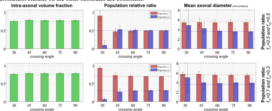
The algorithm provides in fact accurate and precise estimates for crossing angles above 45°; however, as the crossing angle decreases the errors as well as the standard deviations of the estimates with respect to the ground-truth increase. Our results are in line with (and slightly improve) those previously reported by Zhang et al<sup>3</sup>.
