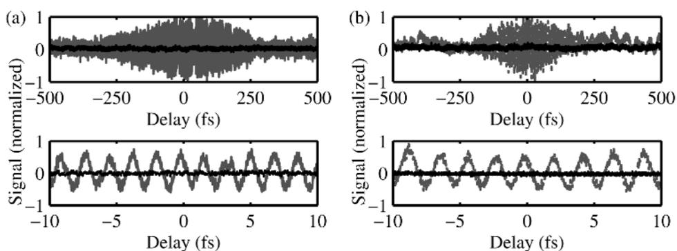
**Fig. 2.** Interferograms showing simultaneous phase coherence between 532-nm and 670-nm OPO outputs and a pump super-continuum. (a) Photodiode signal at 532 nm ( $2s$ ) with locking on (grey) and off (black); (b) photodiode signal at 670 nm ( $p + i$ ) with locking on (grey) and off (black).
