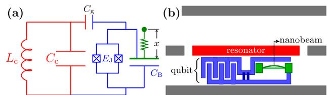
FIG. 1 (color online). (a) Circuit diagram and (b) sketch of the hybrid system composed of a transmon qubit, a superconducting coplanar waveguide resonator, and a mechanical oscillator.
