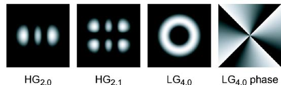
FIG. 1. Hermite-Gaussian (HG) and Laguerre-Gaussian (LG) modes. Shown here are the intensity cross sections of two HG modes,  $HG_{2,0}$  and  $HG_{2,1}$ , and the intensity and phase (gray scale representation) cross sections of one LG mode,  $LG_{4,0}$ , which possesses a central charge-4 vortex.
