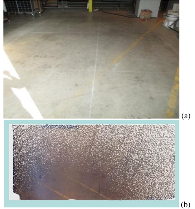
Figure 2. The DL slab (a) and the point cloud associated to its top surface (b)
