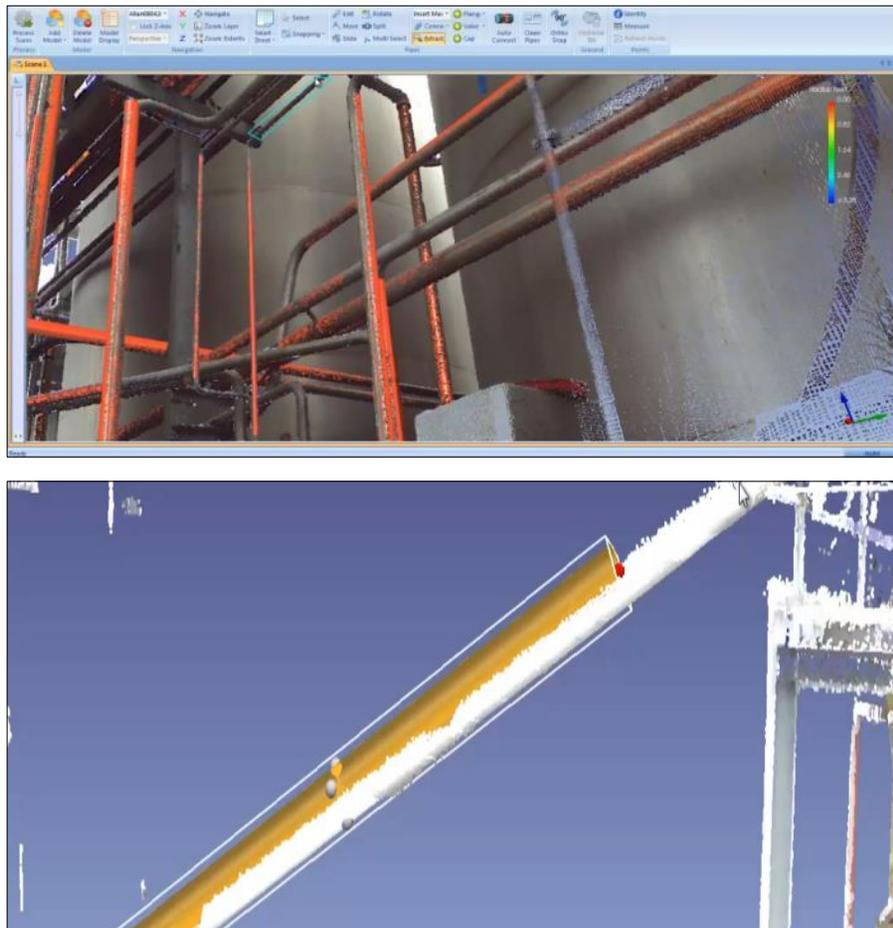
Fig. 4. EdgeWise Plant™ 4.0 by ClearEdge3D
