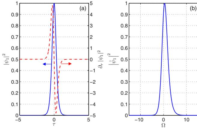
FIG. 1. (Color online) Solid blue curves represent (a) the temporal and (b) the spectral profile of the pump intensity, respectively. Here  $\Omega$  is the normalized frequency shift,  $N = 2.5$ , and  $\tau_{\text{sh}} = 0.1137$ . These parameters are used in all the simulations shown in this paper, except in Fig. 2, where  $N$  is an independent variable. The time derivative of the temporal pulse intensity is shown by the dashed red curve in (a).
