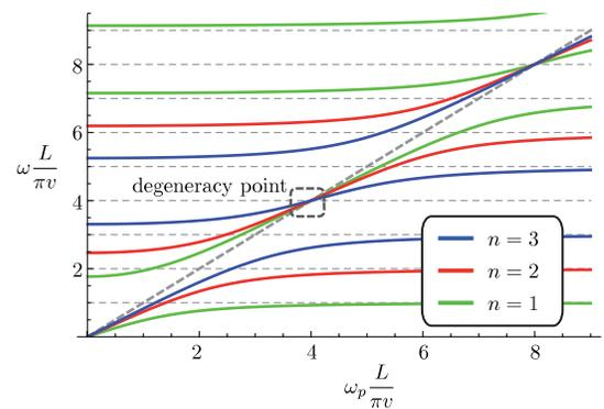
FIG. 2 (color online). Spectrum of CPWR with  $v = 0.98 \times 10^8$  m/s and  $Z_0 = 50\Omega$ , interrupted by three identical and uniformly distributed JJs with  $C_J = 1$  pF and  $L = 28$  mm, plotted over their plasma-frequency  $\omega_p$  in units of the fundamental mode frequency  $(\pi v)/L$ . Eigenmodes of the bare CPWR that do not couple to the JJs are omitted. The dashed box marks the degeneracy point  $\omega_p = \bar{\omega}$ , on which we focus our investigation.
