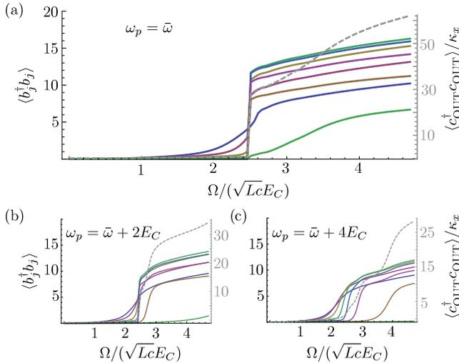
FIG. 3 (color online). Occupancies for the local modes  $b_j$  (colored solid lines) plotted as a function of the drive strength  $\Omega$  (scale at left vertical axes) at the degeneracy point  $\omega_p = \bar{\omega}$  (a) and for plasma frequencies  $\omega_p$  slightly detuned from the degeneracy point (b) and (c). The gray dashed line shows the output intensities (scale at right vertical axes). Parameters:  $v = 0.98 \times 10^8$  m/s,  $Z_0 = 50\Omega$ ,  $C_j = 1$  pF, and  $N = 8$ .
