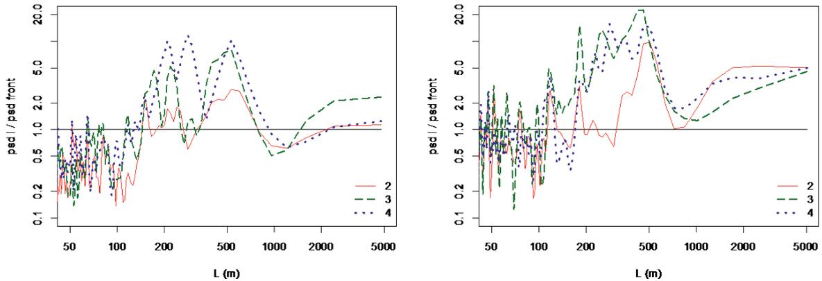
Fig. 6. Ratio of the Spectra of second to fourth turbines over that of the front turbine, with the horizontal axis rescaled to equivalent length scales, (a) at a wind direction of  $223^\circ$  when the all other turbines are fully shaded by the front turbine, and (b) at a wind direction of  $229^\circ$  when the second turbine is only partially shaded by the front turbine.
