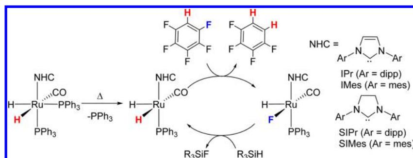
Scheme 2. Mechanisms of Ru-Catalyzed HDF of  $C_6F_5H$  to 1,2,3,4- $C_6F_4H_2$
