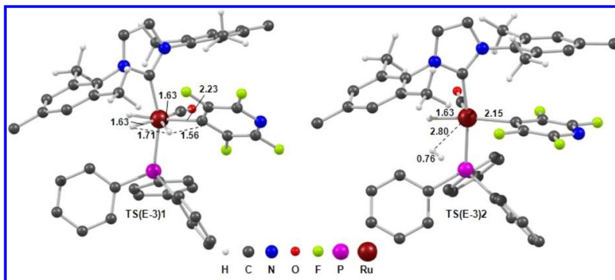
**Figure 6.** Computed structures of TS(E-3)1 and TS(E-3)2 with key distances in Å. PPh<sub>3</sub> and IMes H atoms (with the exception of the IMes *ortho*-Me groups) are omitted for clarity.
