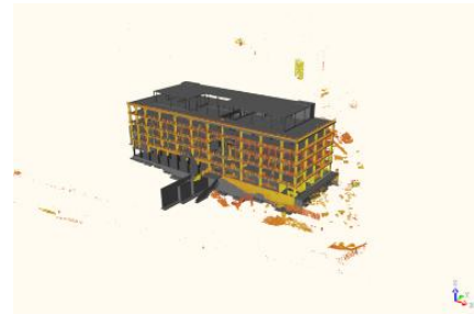
Figure 5 3D model referenced in the scanner's spherical coordinate frame.
