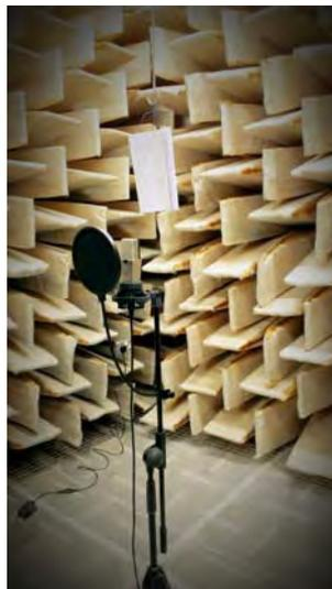
Figure 3 – The setup for voice recording in the anechoic chamber
