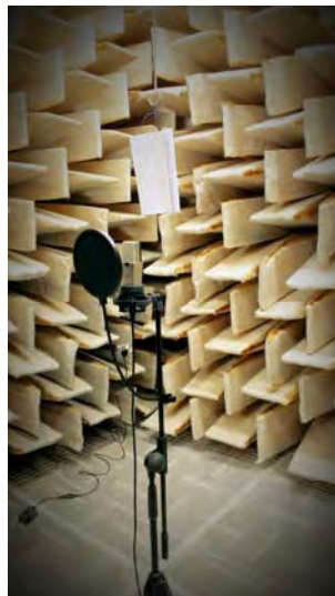
Figure 3 – The setup for voice recording in the anechoic chamber
