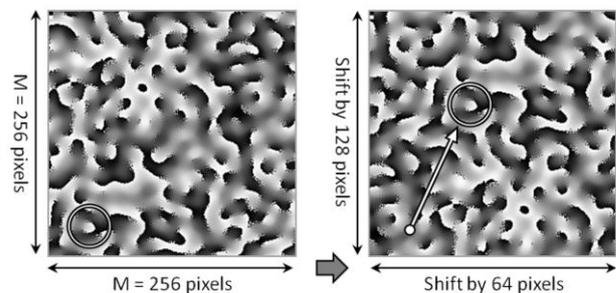
**Fig. 3.** Demonstration of a periodic kinoform shift for a periodicity  $c = 4$ . The CGH is shifted by one period in the horizontal axis and two periods in the vertical axis. The circle tracks a single feature [8].
