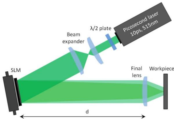
**Fig. 1.** Schematic diagram of the optical setup used in laser marking experiments.
