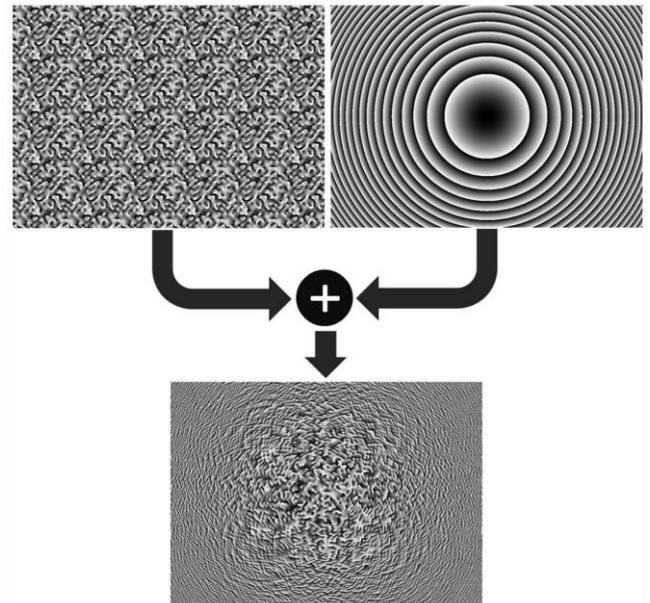
**Fig. 2.** Generation process of the CGH with the software-written FZL.
