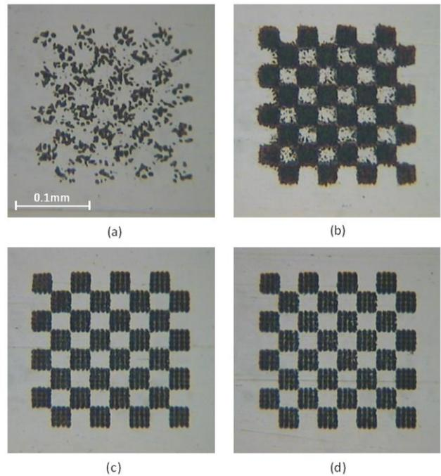
**Fig. 6.** Checkerboard pattern produced by using four different approaches: (a) basic approach, (b) time-averaging technique, (c) our new laser-marking approach, and (d) an alternative approach to (c). Patterns (a) and (b) were generated at  $P = 7.1$  W, while patterns (c) and (d) were produced at  $P = 2.25$  W.
