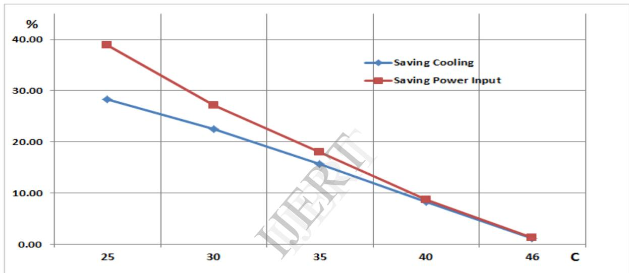
Figure6. Cooling capacity and power input saving (%)
