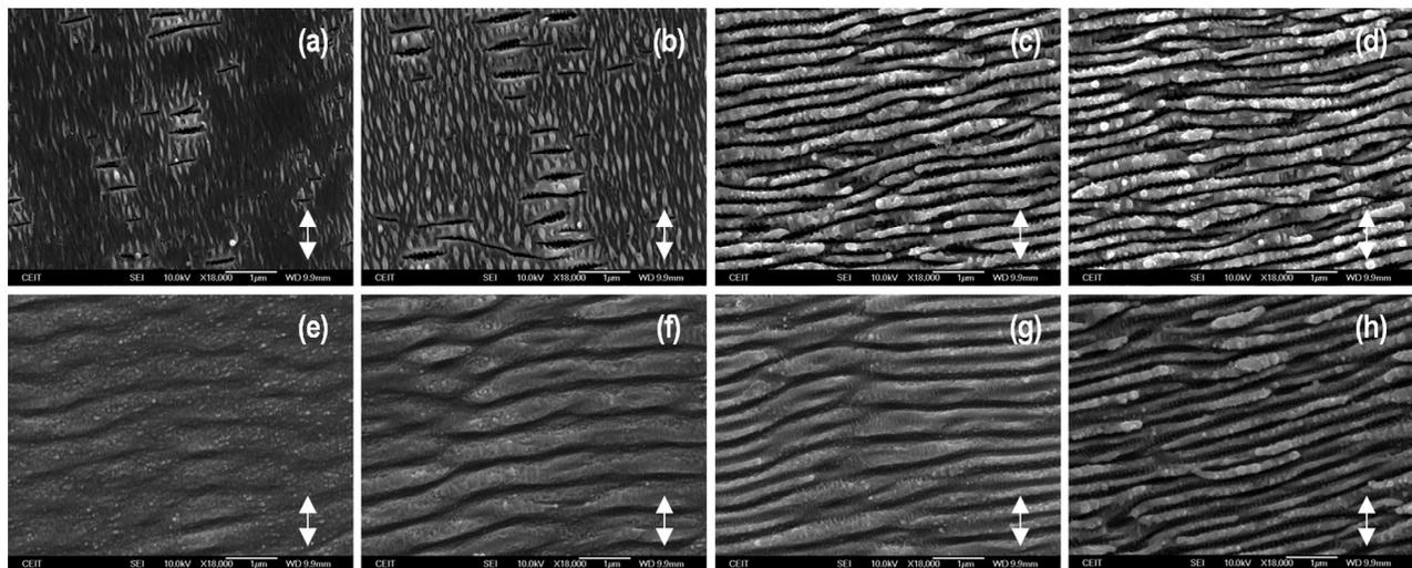
FIG. 2. FESEM images of the Nb surface after laser irradiation at fluences of  $29 \text{ mJ}\cdot\text{cm}^{-2}$  from (a) to (d) and  $53 \text{ mJ}\cdot\text{cm}^{-2}$  from (e) to (h). The number of pulses applied are (a) 1139, (b) 1898, (c) 3796, (d) 5694 pulses, (e) 85, (f) 142, (g) 284, and (h) 851 pulses. The arrow shows the polarization of the incident laser beam.
