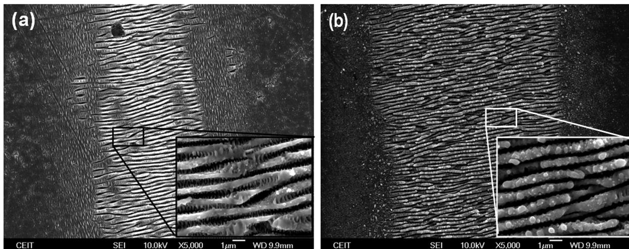
FIG. 4. FESEM micrographs of Niobium samples irradiated at (a) 32 mJ·cm<sup>-2</sup> and 0.1 mm·s<sup>-1</sup> (1087 pulses) and (b) 32 mJ·cm<sup>-2</sup> and 0.03 mm·s<sup>-1</sup> (3623 pulses). The insets show images at 18000× magnification of the central area.
