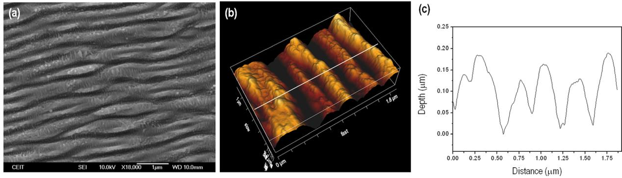
FIG. 7. AFM analysis of Niobium surface after femtosecond laser irradiation at  $47 \text{ mJ}\cdot\text{cm}^{-2}$  and  $0.3 \text{ mm}\cdot\text{s}^{-1}$  (302 pulses). (a) FESEM micrograph; (b) higher magnification AFM 3D image of (a); and (c) cross section profile by the line showed on (b).
