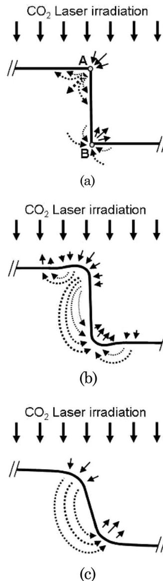
Fig. 1. Surface relaxation of the etched structure by  $\text{CO}_2$  laser irradiation. Solid arrows indicate the significant pressure acting on the molten edges, whereas dotted arrows indicate the liquid flow.
