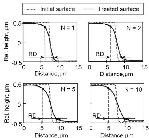
Fig. 3. Evolution of the step profile of the binary grating as a function of laser line scans,  $N$ , with fixed laser power,  $P = 7.35\ \text{W}$ . The diameter of the laser beam was  $\sim 1\ \text{mm}$ .
