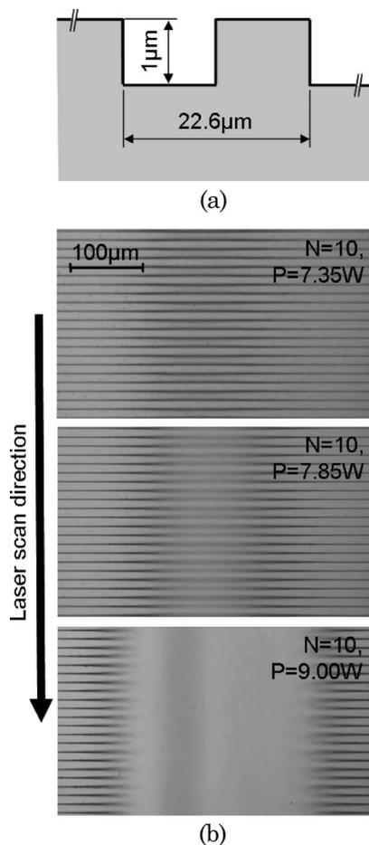
Fig. 2. (a) Illustration of the binary grating with spatial period of  $22.6\ \mu\text{m}$  and step height of  $1\ \mu\text{m}$ . (b) Micrographs of the structure after laser treatment with  $N = 10$  unidirectional scans in the direction shown, for laser power of  $7.35\ \text{W}$ ,  $7.85\ \text{W}$ , and  $9.00\ \text{W}$ , respectively.
