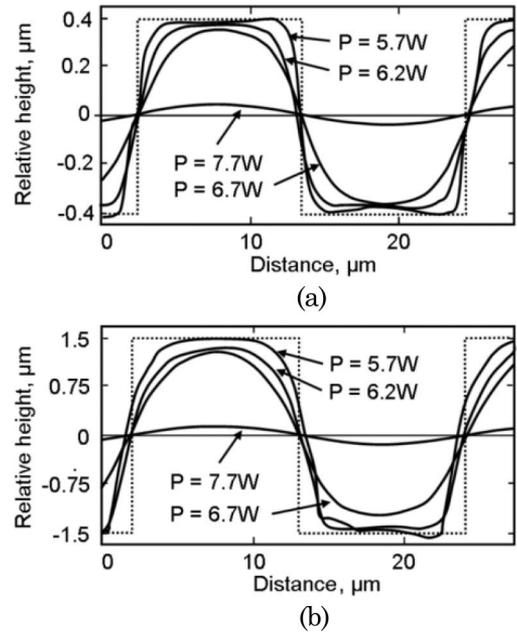
Fig. 4. AFM surface profile of laser-treated binary samples with (a) 0.8  $\mu\text{m}$  initial step height and (b) 3  $\mu\text{m}$  initial step height. Dotted line indicates ideal shape of a binary grating before laser smoothing. The diameter of the laser beam used was  $\sim 550 \mu\text{m}$ .
