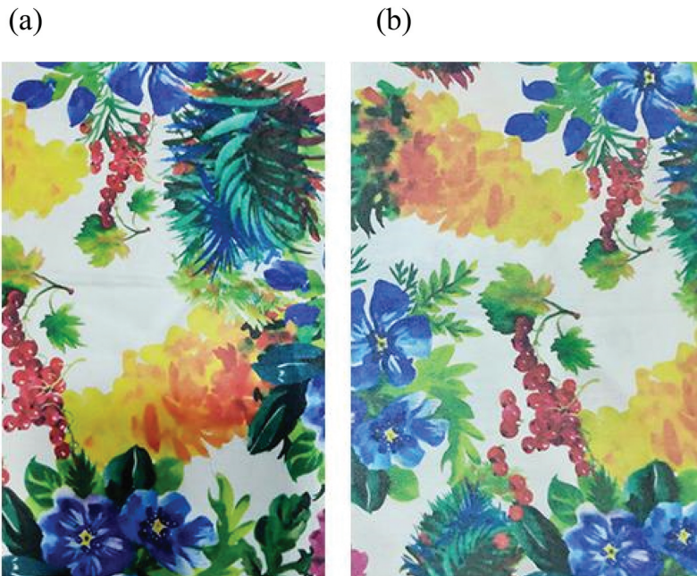
Figure 1. The difference in print quality in-between (a) Pre-treated fabric and (b) No pre-treated fabric after inkjet printing (Splashjet Inkjet Ink Private Limited 2020).
