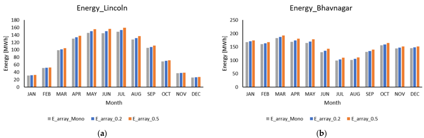
Figure 4. Monthly energy generation of the (a) Lincoln Solar Farm and (b) Bhavnagar Solar Farm.
