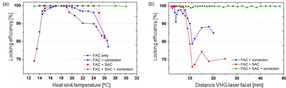
Fig. 3. Efficiency of VHG locking with DE = 15% (a) as a function of temperature of the heat sink with VHG placed at 3 mm distance from the laser and (b) distance between the VHG and laser facet for 0.6 nm VHG offset.
