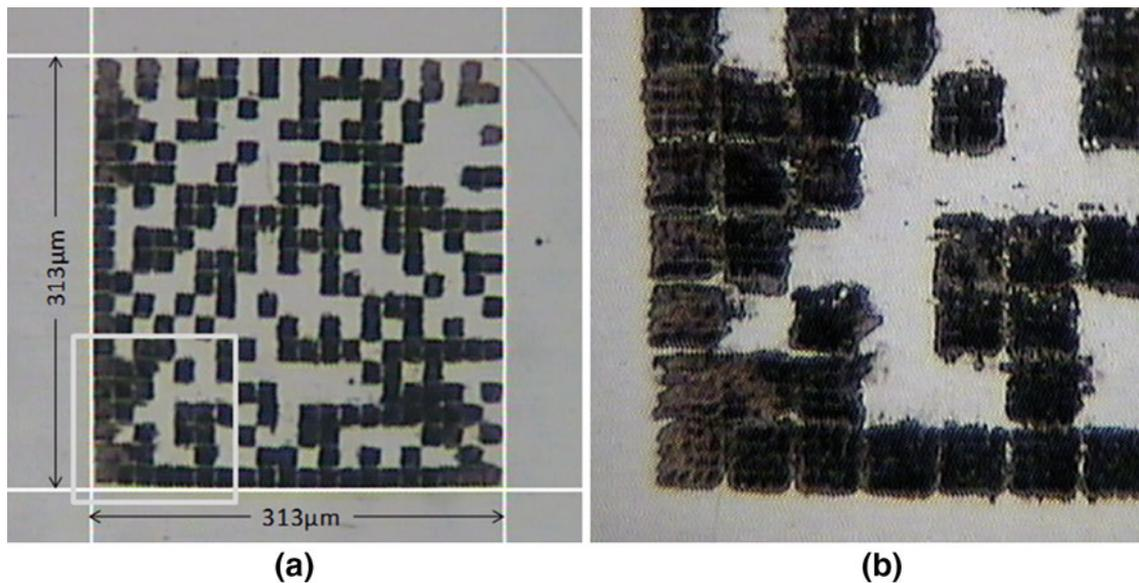
**Fig. 6** **a** Datamatrix containing a code with 22 alphanumeric characters. This datamatrix was produced on the surface of Chromflex steel using our invented laser-marking method at  $P = 10.9$  W. **b** Close-up view of the left-bottom corner of the datamatrix shown in **a**
