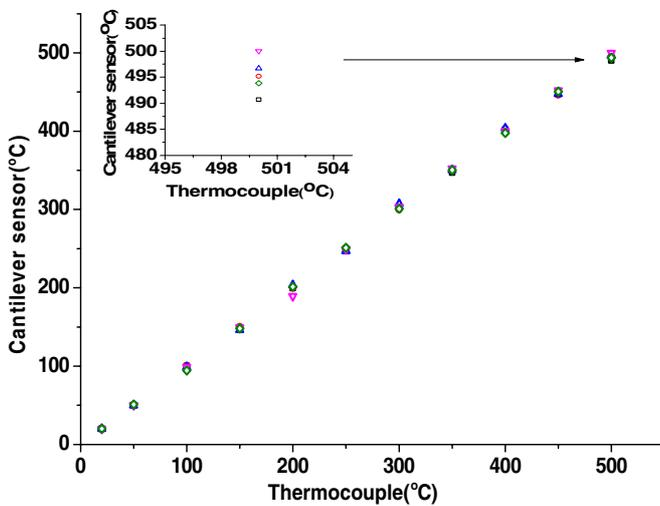
Figure 9. Monitored temperature versus cantilever thermal sensor.
