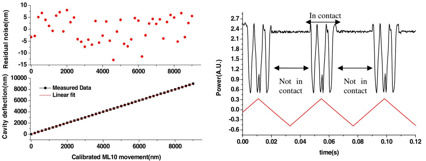
**Figure 4.** (a) Measured cavity length versus movement of ML10. (b) Dynamic response of micro-machined cantilever: top trace shows return from the cavity monitored at a single wavelength, bottom trace shows the piezo driving voltage which will approximate the piezo stage displacement.
