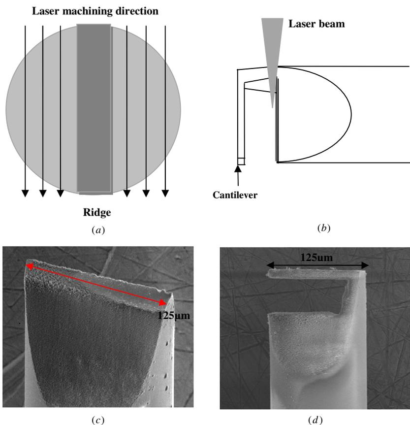
**Figure 1.** Outline laser machining process to form fibre-top cantilever, (a) ps-laser machine a ridge onto cleaved fibre (top view), (b) ps-laser under-cut to form free standing cantilever (side view), (c) SEM view of machined ridge and (d) SEM view of ps-laser machined cantilever.
