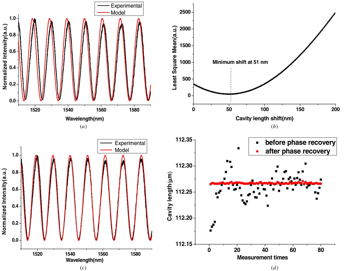
**Figure 5.** (a) Experimental spectrum and model based on starting cavity length recovered from FFT algorithm. (b) Plot of least mean squares fit between experimental and modelled data versus a small shift in cavity length around the FFT value. (c) Comparison between model and experimental after phase recover process applied. (d) Noise measurement over 80 scans for a stabilized cavity length before and after phase recovery algorithm.
