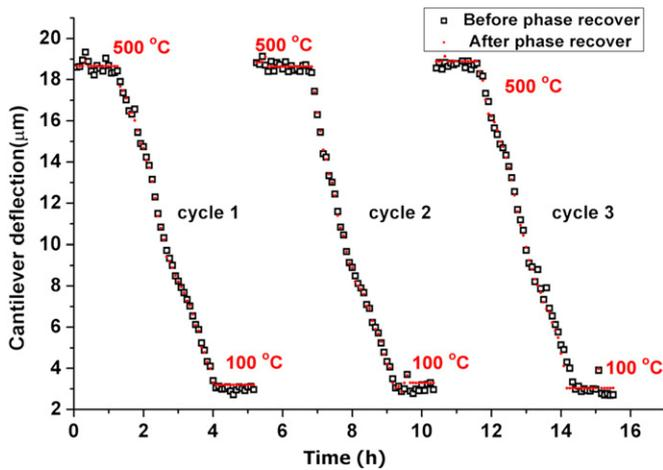
Figure 8. Cantilever deflection versus cooling time.
