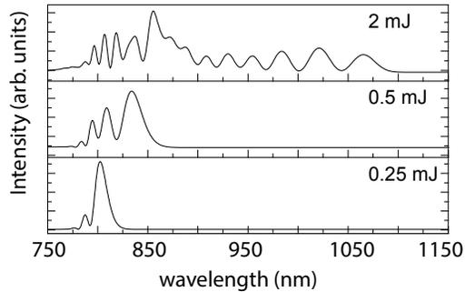
Fig. 2. Numerically simulated spectra with different input pulse energies from the 700  $\mu\text{m}$  core fiber with internal silver and polymer coating (fiber E) assuming 100% Raman contribution to the nonlinearity.
