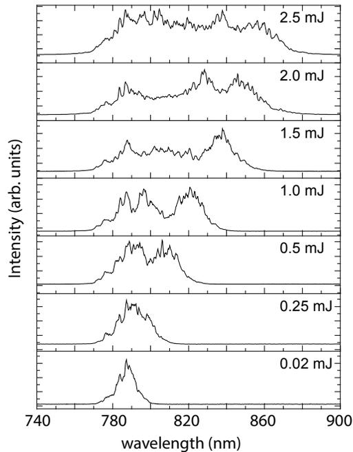
Fig. 1. Experimentally measured spectra with different input pulse energies from the 700  $\mu\text{m}$  core fiber with internal silver and polymer coating (fiber E). The transform limited pulse duration of these spectra vs. input pulse energy is 78, 56, 36, 28, 21, 20, 19 fs for 0.02, 0.25, 0.5, 1.0, 1.5, 2.0, 2.5 mJ input energy. All fibers investigated delivered very similar spectra.
