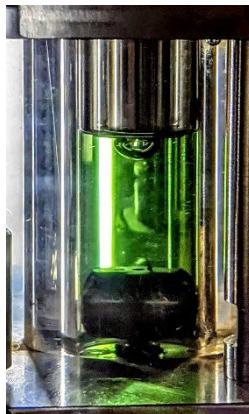
Figure 4: Picture of the cell with the \text{CO}_2 + \text{N}_2\text{O}_4 mixture at low temperature
