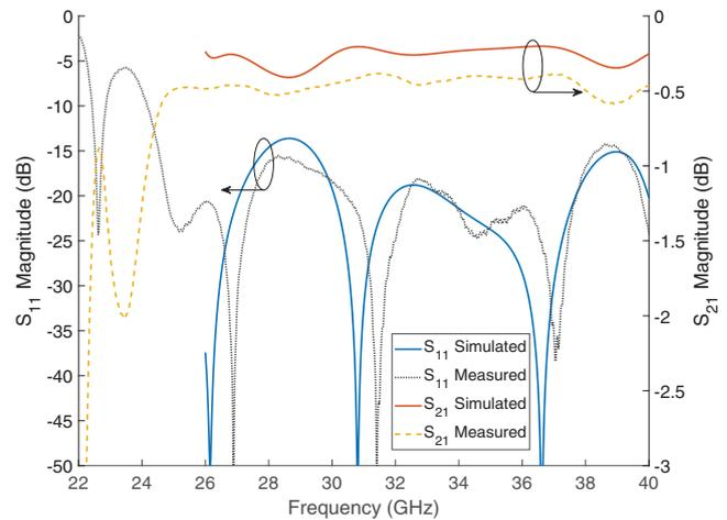
Fig. 6 Simulated and measured results of the back-to-back structure
