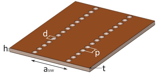
Fig. 2 SIW geometry
