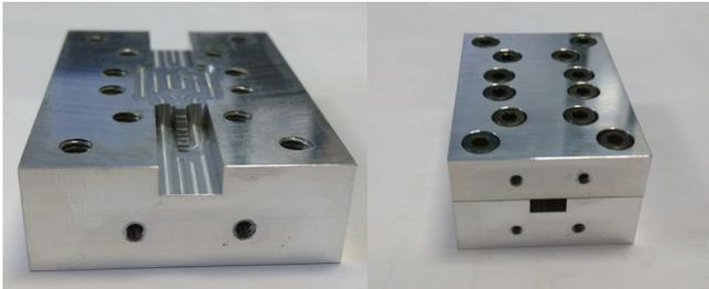
Fig. 4 Photo of the manufactured back-to-back transition prototype
