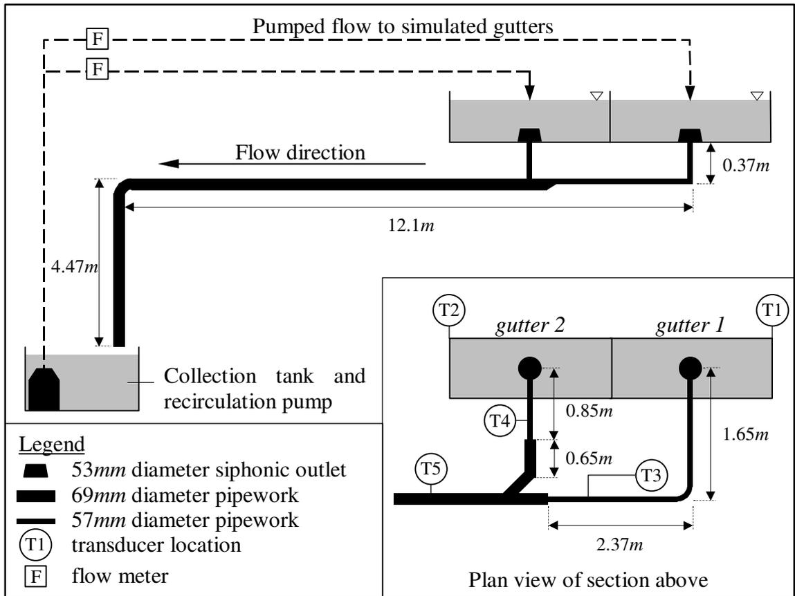
**Figure 2: Schematic view of the siphonic roof drainage test rig. The capacity of the system is the same as 75mm/hour falling on a 665m<sup>2</sup> roof – all drained via a 69mm diameter pipe.**
