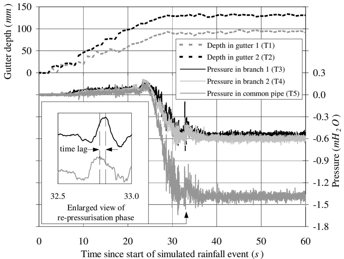
**Figure 4: Measured gutter depths and system pressures for the design criteria rainfall event (*gutter 1* inflow = 5.85l/s, *gutter 2* inflow = 7.78l/s). These data illustrates that even when fully primed (40-60 seconds) the pressures are not truly “steady”.**
