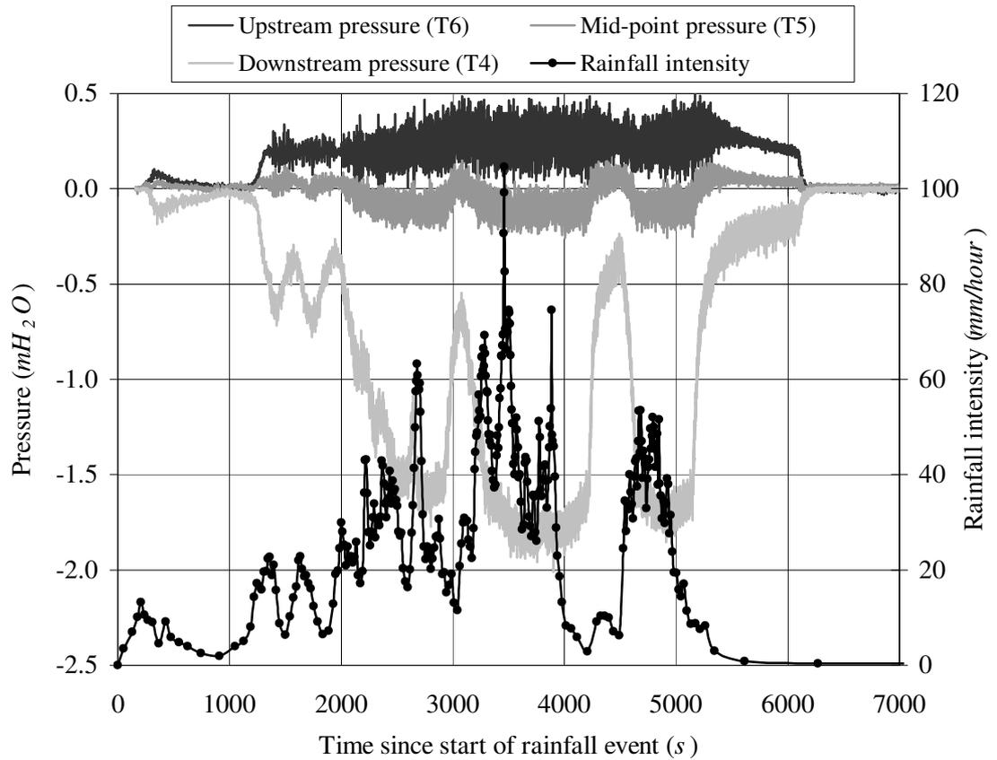
**Figure 10: Measured conditions (*system 2*) on 2<sup>nd</sup> August 2000 (refer to Figure 9 for system and transducer layout). The time varying nature of this rainfall event is typical, and demonstrates the importance of using rainfall hietographs to fully assess system performance.**
