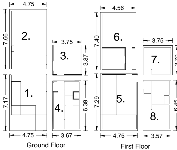
Fig. 1. The modular precast villa of eight boxes designed by DuBox.
