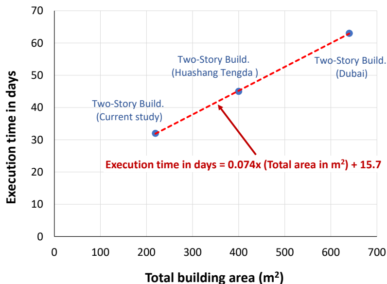
Fig. 5. Relationship between the total area of the building and the execution time for two-storey 3DCP buildings.
