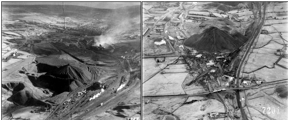
129 Figure 2: Legacy stockpiles of slag materials at Blaenavon ironworks during active operation 130 (Aerial images reproduced, courtesy Welsh Government Aerial Photographs Unit).
