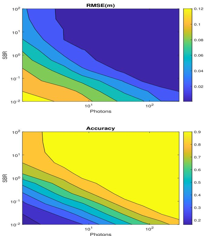
Fig. 3. Depth RMSEs (up) and Classification accuracy (down) of the subsampled lego data ( $N = 40 \times 40$ ,  $T = 1500$ ,  $L = 4$ ,  $K = 3$ ) w.r.t. signal-to-background ratio (SBR) and the average signal photons per pixel and per wavelength.
