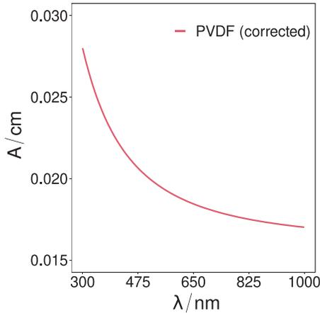
**Fig. 6.** The determined optical absorbance coefficients of the PVDF sample over the spectral range of 300 nm to 1000 nm, as calculated from the corrected transmissivity intensity.
