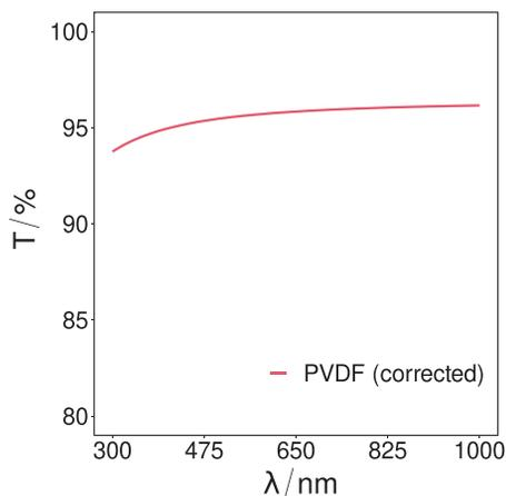
**Fig. 4.** The corrected transmissivity intensity of the PVDF sample over the spectral range of 300 nm to 1000 nm. The mean transmissivity over the spectrum is determined to be  $(95.6 \pm 0.6)\%$ .
