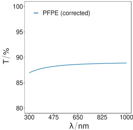
**Fig. 3.** The corrected transmissivity intensity of the PFPE sample over the spectral range of 300 nm to 1000 nm. The mean transmissivity over the spectrum is determined to be  $(88.4 \pm 0.5)\%$ .
