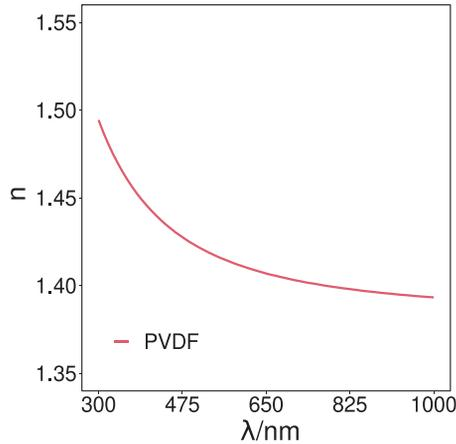
**Fig. 2.** The ellipsometric (real) indices of refraction ( $n$ ) values of the PVDF sample over the spectral range of 300 nm–1000 nm. Data derived from the Cauchy optical model using the Levenberg-Marquardt fitting algorithm. The refractive index was found to be 1.41 ( $\lambda = 589.3$  nm).
