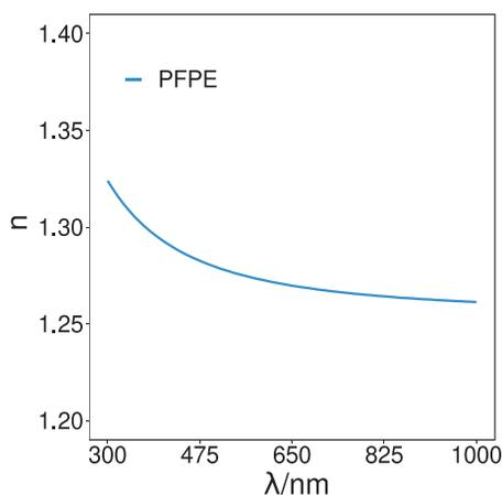
**Fig. 1.** The ellipsometric (real) indices of refraction ( $n$ ) values of the PFPE sample over the spectral range of 300 nm–1000 nm. Data derived from the Cauchy optical model using the Levenberg-Marquardt fitting algorithm. The refractive index was found to be 1.27 ( $\lambda = 589.3$  nm).
