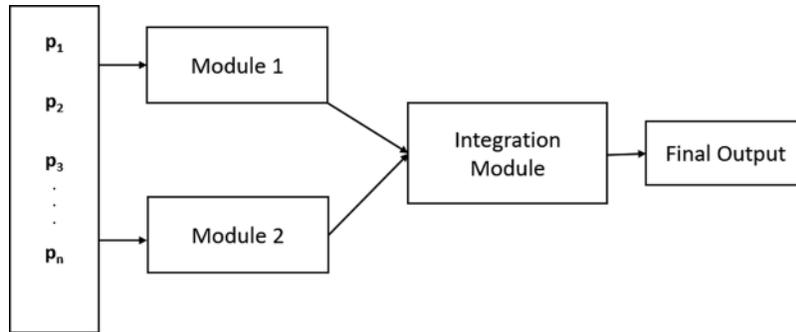
**Figure 4:** Modular neural network with 2 modules
