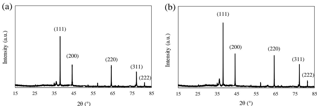
Fig. 6 XRD patterns of the Ag NPs. (a) Hotplate-based method, 300°C, 30 min. (b) Laser-based method, 70 W, 5 min.
