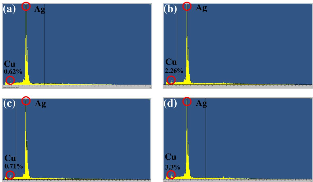
Fig. 5. EDS results of the fracture surfaces of the Si-Ag-DBC joints. (a) Hotplate-based method, 300°C, 30 min, 0.3 MPa; (b) Hotplate-based method, 300°C, 30 min, 3.0 MPa; (c) Laser-based method, 70 W, 1 min, 3.0 MPa; (d) Laser-based method, 70 W, 5 min, 3.0 MPa.
