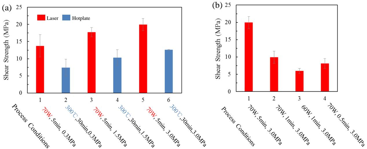
Fig. 2. Measurement results of the shear strength. (a) Comparison of shear strength of different sintering methods and pressures. Process conditions: 1. 70 W, 5 min, 0.3 MPa; 2. 300°C, 30 min, 0.3 MPa; 3. 70 W, 5 min, 1.5 MPa; 4. 300°C, 30 min, 1.5 MPa; 5. 70 W, 5 min, 3.0 MPa; 6. 300°C, 30 min, 3.0 MPa. (b) Comparison of shear strength of different laser powers and times. Process conditions: 1. 70 W, 5 min, 3.0 MPa; 2. 70 W, 1 min, 3.0 MPa; 3. 60 W, 1 min, 3.0 MPa; 4. 70 W, 0.5 min, 3.0 MPa.
