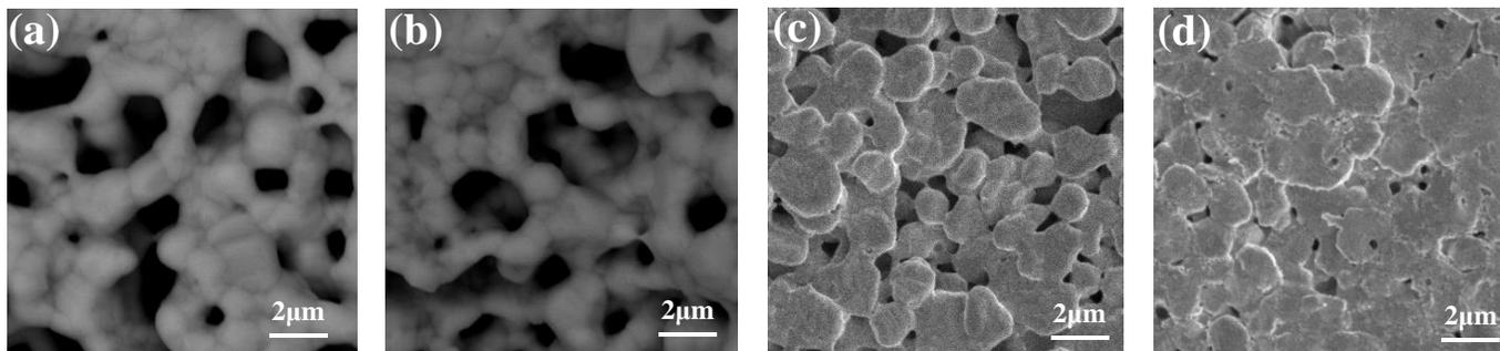
Fig. 4. SEM images of the fracture surfaces of the Si-Ag-DBC joints. (a) Hotplate-based method, 300°C, 30 min, 0.3 MPa; (b) Hotplate-based method, 300°C, 30 min, 3.0 MPa; (c) Laser-based method, 70 W, 5 min, 0.3 MPa; (d) Laser-based method, 70 W, 5 min, 3.0 MPa.
