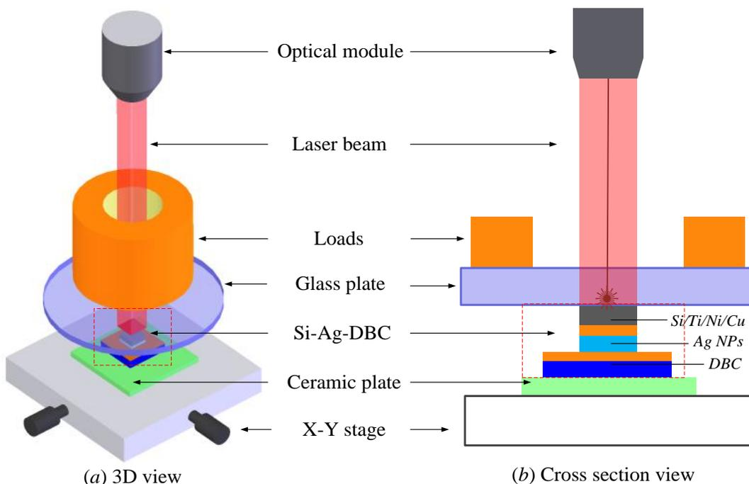
Fig. 1. Schematic of the laser-based sintering setup. (a) 3D view and (b) Cross-sectional view.
