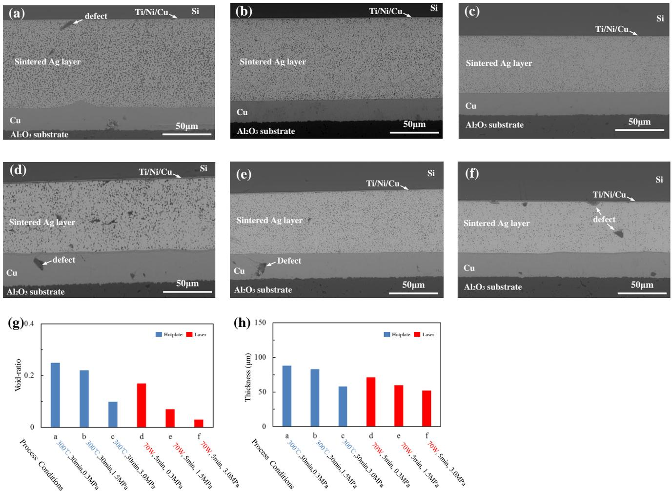
Fig. 3. SEM images of cross-sections of the Si-Ag-DBC joints. (a) Hotplate-based method, 300°C, 30 min, 0.3 MPa; (b)
