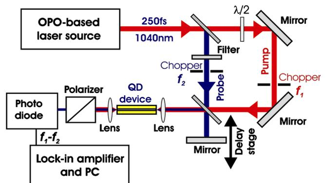
FIG. 1. (Color online) Schematic of the DTS setup.
