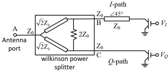
Fig. 1. Dual-transistor based IQ backscatter modulator.
