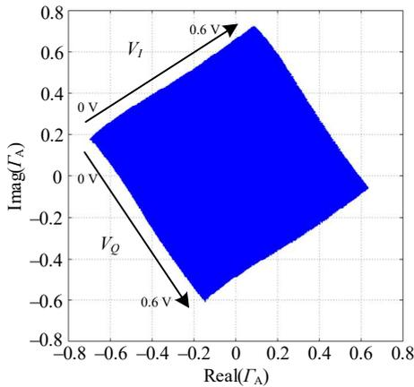
Fig. 2. Reflection coefficient observed at antenna port A when  $V_I$  and  $V_Q$  of two transistors (ATF-54143) are swept from 0 to 0.6 V. Measured Transistor impedance at 2.45 GHz and an ideal Wilkinson power splitter are used for the plot.
