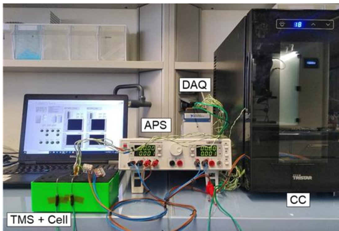
Figure 1: Experimental Test Rig at HSLU, as employed in [4]. Legend: TMS=Thermal Management System, APS=Arbitrary Power Supply, DAQ=Data Acquisition system, CC=Cooling Chamber.
