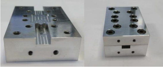
Fig. 4 Photo of the manufactured back-to-back transition prototype.
