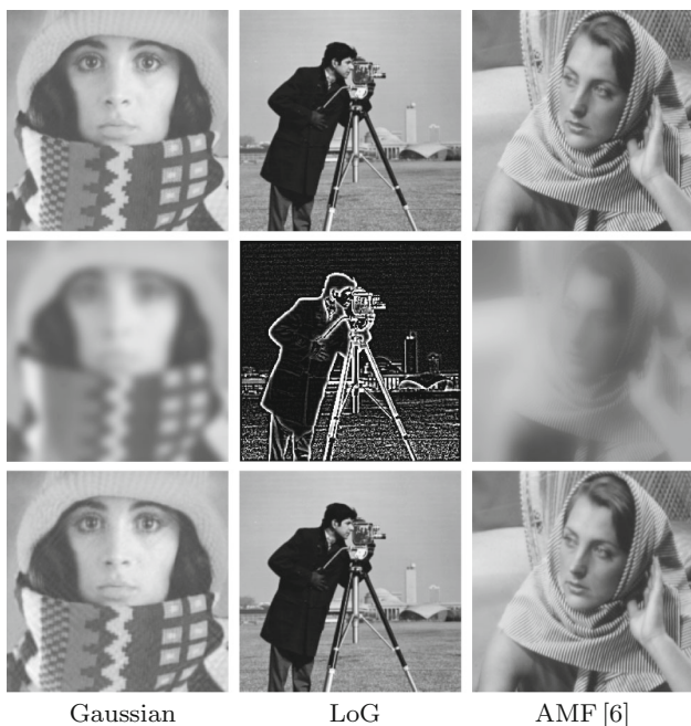
Fig. 1 Top row: test images we deal with in this paper: Trui, cameraman, and Barbara. Middle row: the images are filtered by a Gaussian imgaussfilt(x,5) , Laplace-of-Gaussian imfilter(x,fspecial('log',7,0.4)) , and the adaptive manifold filter (AMF) adaptive_manifold_filter(x,20,0.4) [6], respectively (Matlab notations are used to specify the parameters of the filters). Bottom row: defiltering results; notice how well the fine image details are restored
