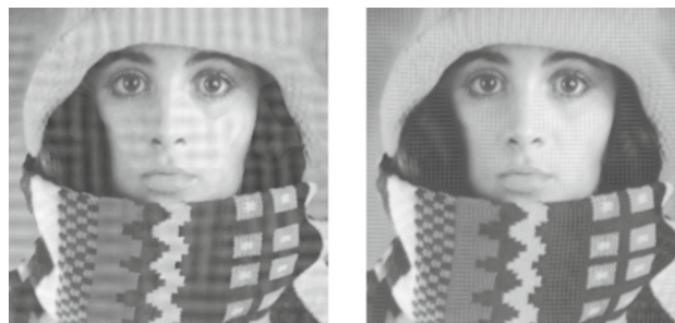
Fig. 7 Overrestoration examples. Left: WMF defiltering with 100 iterations of (4) amplifies certain middle-range frequencies. Right: BF defiltering with 1K iterations of (4) amplifies some high frequencies. Compare these results with those for WMF and BF from Figures 5 and 6, respectively
