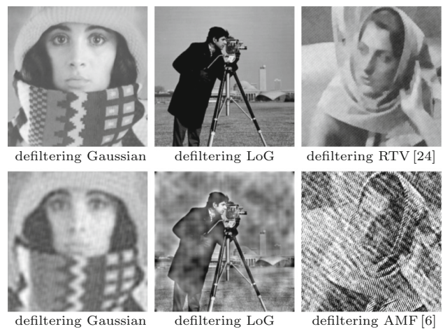
Fig. 4 Defiltering imgaussfilt(x, 5, 'Padding', 'circular') (top-left) and imgaussfilt(x, 5) (bottom-left) by (7). Similar defiltering results for imfilter(x, fspecial('log', 7, 0.4)) with (top-middle) and without (bottom-middle) periodic boundary conditions by (7). Top-right: defiltering RTV [24] with default settings by (7). Bottom-right: defiltering AMF [6] adaptive_manifold_filter(x, 20, 0.4) by (7)
