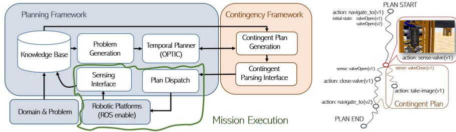
**Fig. 2.** System architecture supporting temporal and contingent planning (left) and a temporal contingent plan solution based on possible valve states (right).
