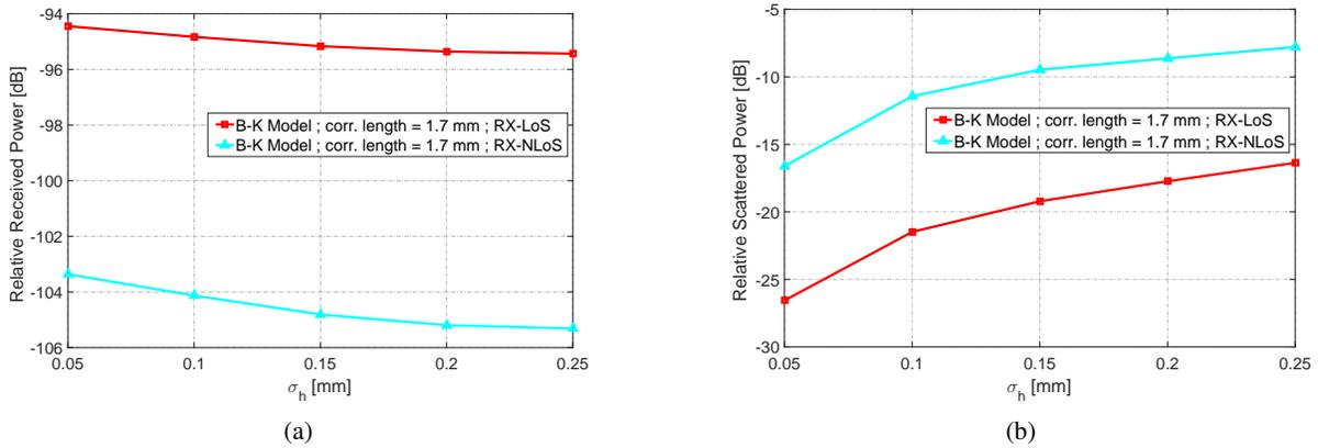
Fig. 1: B-K model at 300 GHz for different roughness parameters for RX-LoS and RX-NLoS receiver locations (a) Total received power relative to input power and (b) Scattered power relative to total received power.
