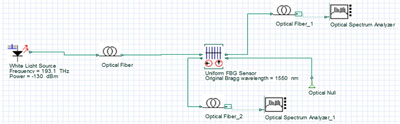
Figure 2: Arrangement of FBG setting.
