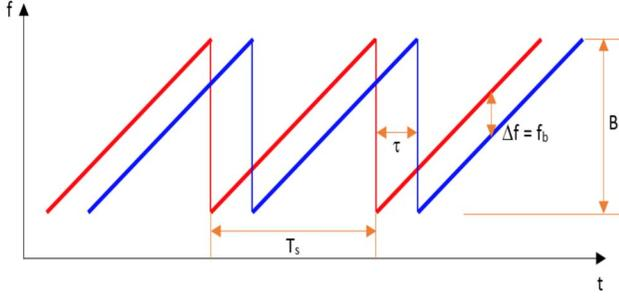
Fig. 4 “Sawtooth” mode of transmitted and received signals from the radar module, where  $f$ = frequency,  $t$ = time,  $T_s$  = sweep duration,  $\tau$  = two way travel time of return signal,  $B$  = sweep bandwidth and  $\Delta f$ = intermediate frequency [21]
