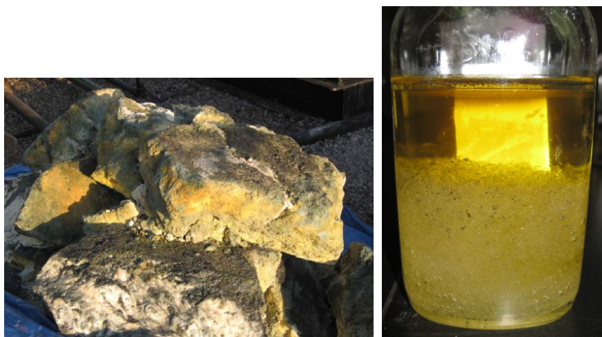
25 26 27 28 29 30 31 32 33 34 35 36 37 Figure 8 – (left) example of amorphous polymeric dithiazine deposition in field installations, note the 38 very pervasive and solid form; and, (right) crystallization of monomeric dithiazine which will remain in 39 this form for only a few hours before spontaneously polymerizing to form apDTZ 36 40 41 42
