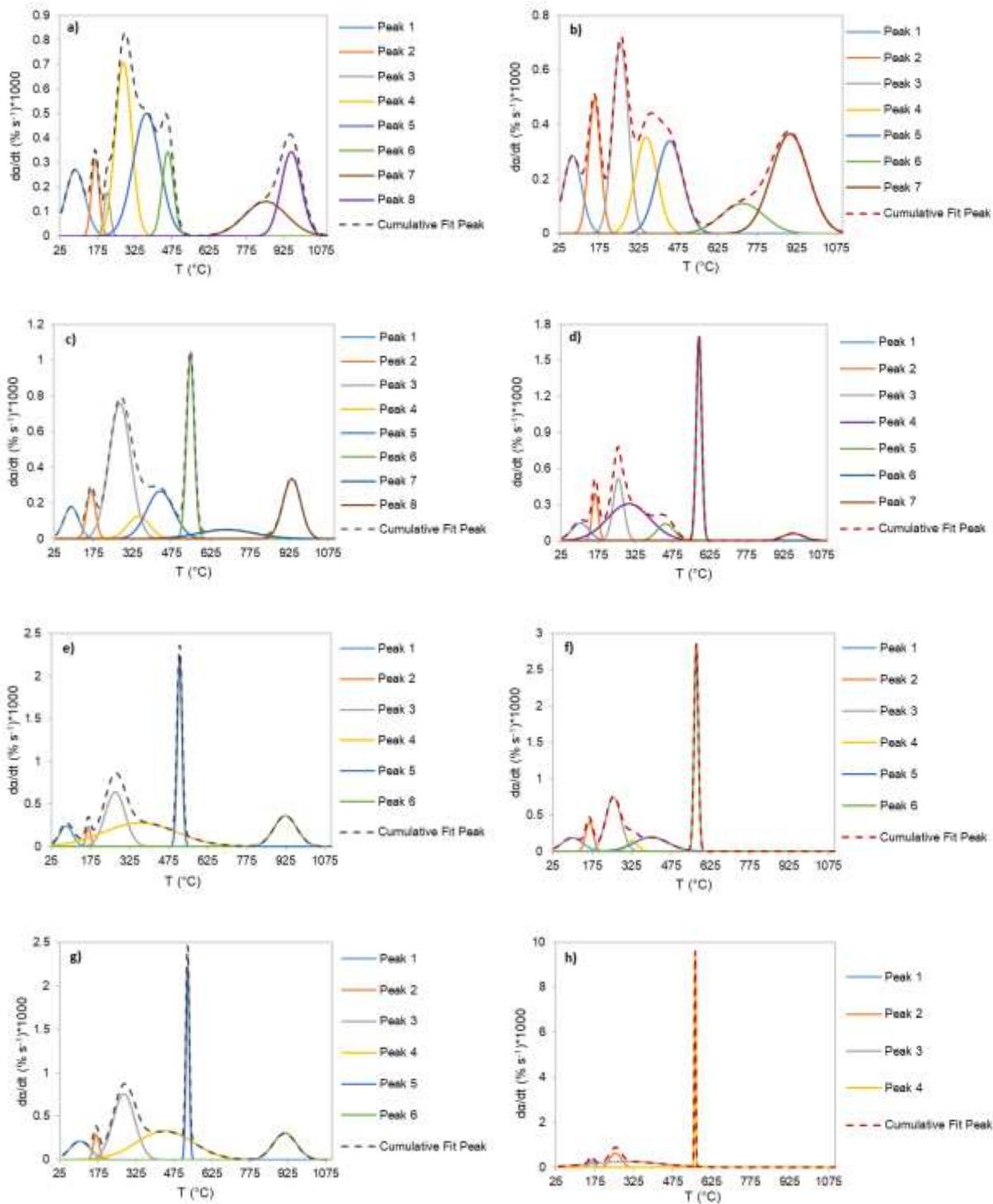
Figure 5. Comparison between the cumulative and estimated curves of each pseudo-component of Na (left side) and Te (right side), respectively, at 20 °C/min in
