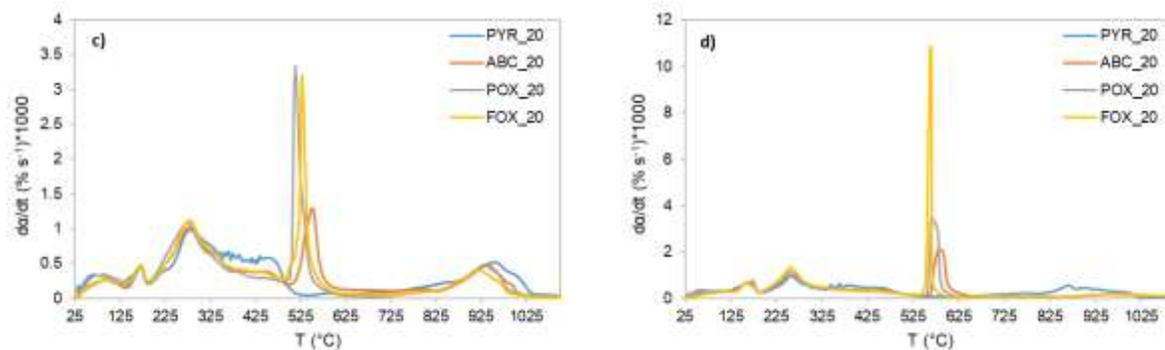
Figure 1. TG (a and b) and DTG curves (c and d) of Na (left side) and Te (right side), at 20 °C/min.
