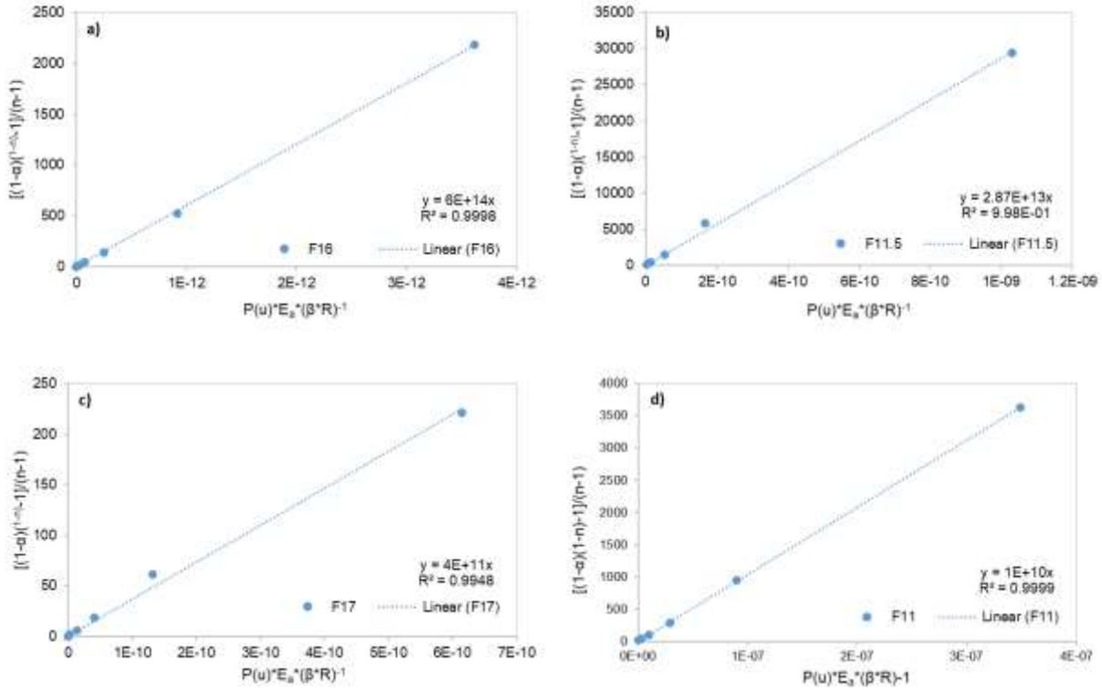
Figure 4. Plots of  $g(\alpha) = [(1-\alpha)^{(1-n)} - 1]/(n-1)$  versus  $P(u)E_a/(\beta R)$  between  $0.05 \leq \alpha \leq 0.5$  and  $0.5 \leq \alpha \leq 0.7$  for Na (a and b), and between  $0.05 \leq \alpha \leq 0.4$  and  $0.4 \leq \alpha \leq 0.65$  for Te (c and d) in pyrolysis process at  $\beta=20$ °C/min.
