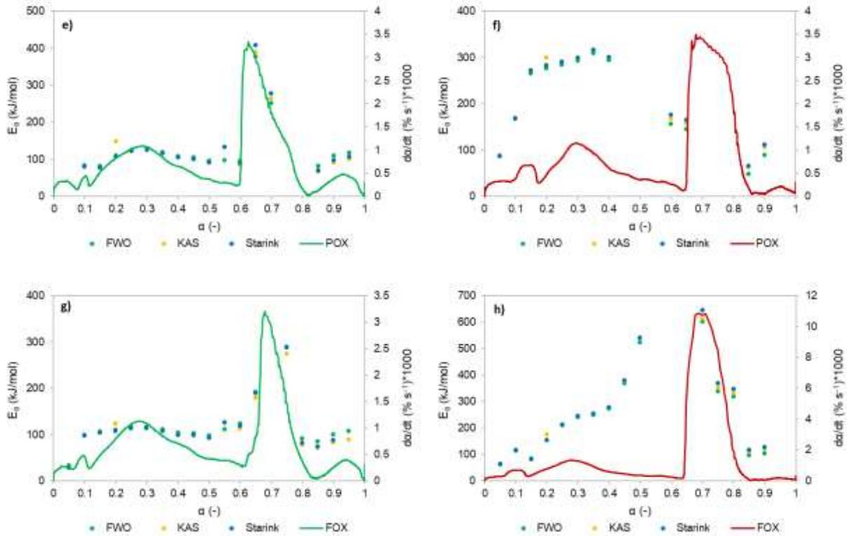
Figure 2. Comparison between activation energy, calculated by FWO, KAS and Starink method, and conversion rate of Na (left side) and Te (right side) in pyrolysis (a and b), combustion (c and d), partial oxy-combustion (e and f) and full oxy-combustion (g and h) processes, at 20 °C/min.
