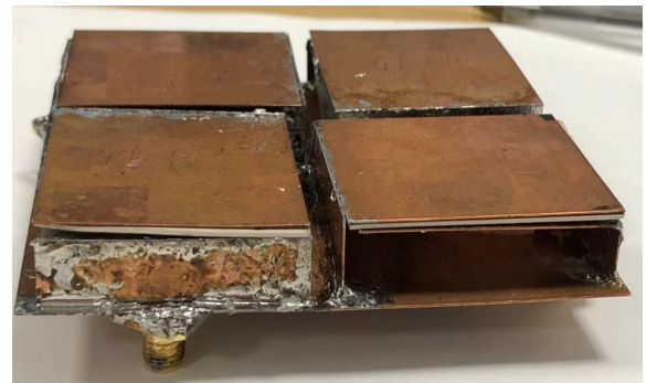
Fig. 10. Perspective view of the fabricated FSP array.
