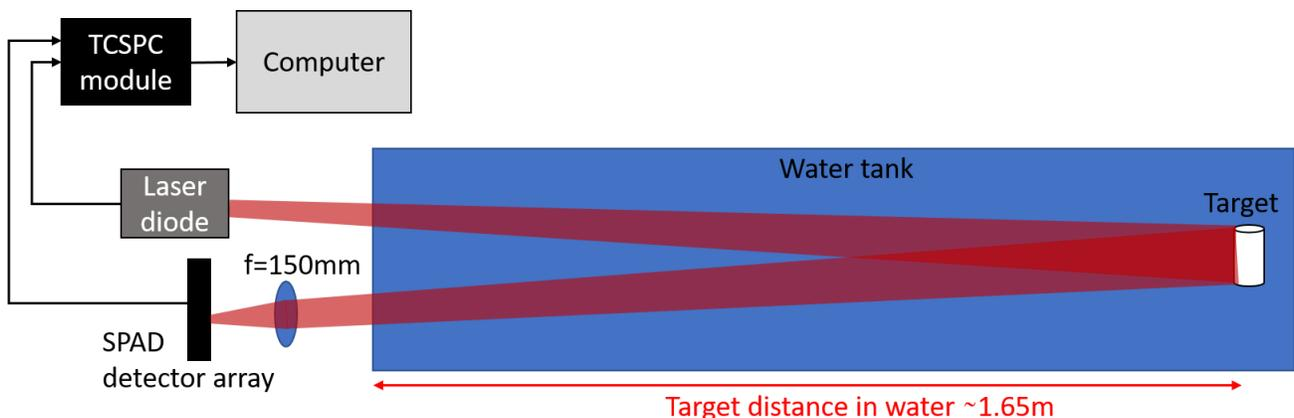
**Figure 1. Schematic of the experimental setup. The system comprised a laser diode, a SPAD detector linear array, and a dedicated TSCPC module. A target was placed in water and the scan was performed by moving the target over the vertical direction.**
