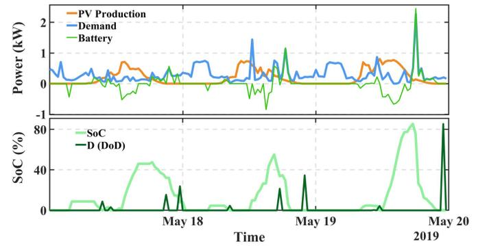
Fig. 3. Example of optimization outputs, with the variable  $D$  accurately capturing the DoD of each discharging half-cycle.
