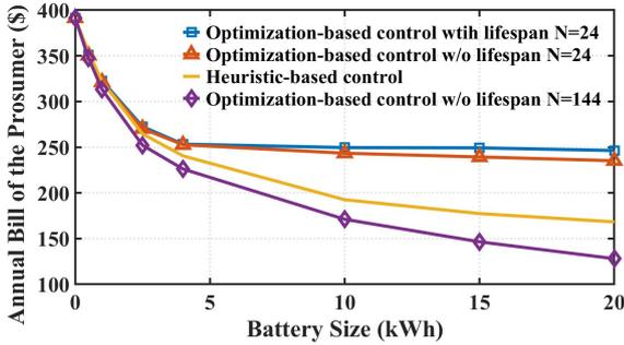
Fig. 4. Comparison of the annual bill achieved with the different control algorithms for batteries capacities ranging from 0 to 20 kWh.
