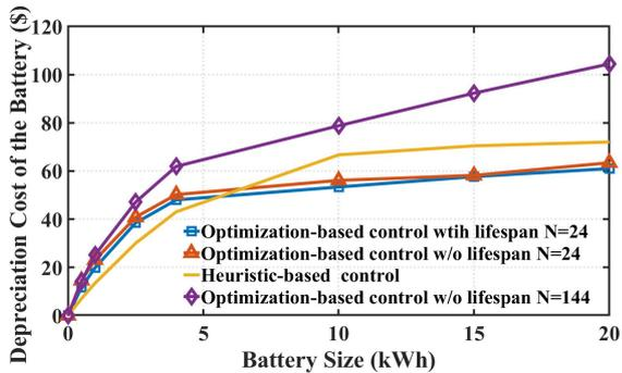
Fig. 5. Annual cost for the depreciation of the battery for the different control algorithms and for different battery capacities.
