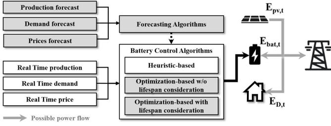
Fig. 1. Schematic of battery control algorithms used in this study
