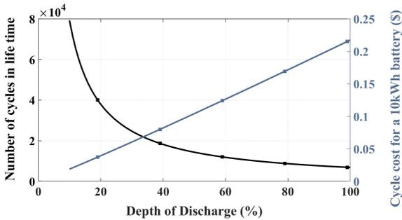
Fig. 2. Allowed number of cycles in a battery life time (right) and the cost associated with a cycle of a certain DoD for a 10 kWh battery, using a battery cost of 250\$/kWh
