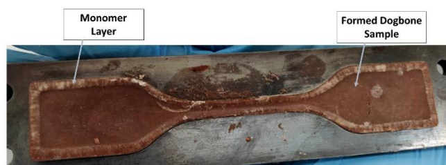
Fig. 5. The formed nanocomposite sample using the infusion method syringe setup.
