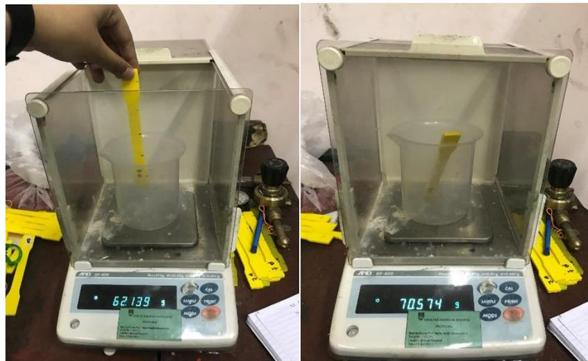
**Figure 5.** Weight of the specimen measured using an electronic scale.
