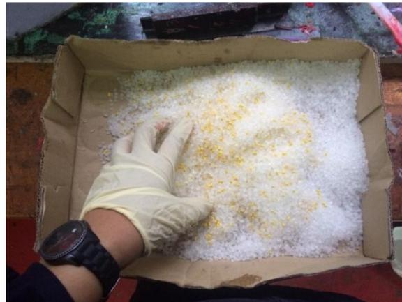
**Figure 2.** Polypropylene and master batch hand mixed.
