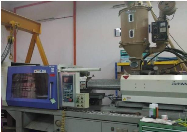
**Figure 1.** Injection Moulding Machine
